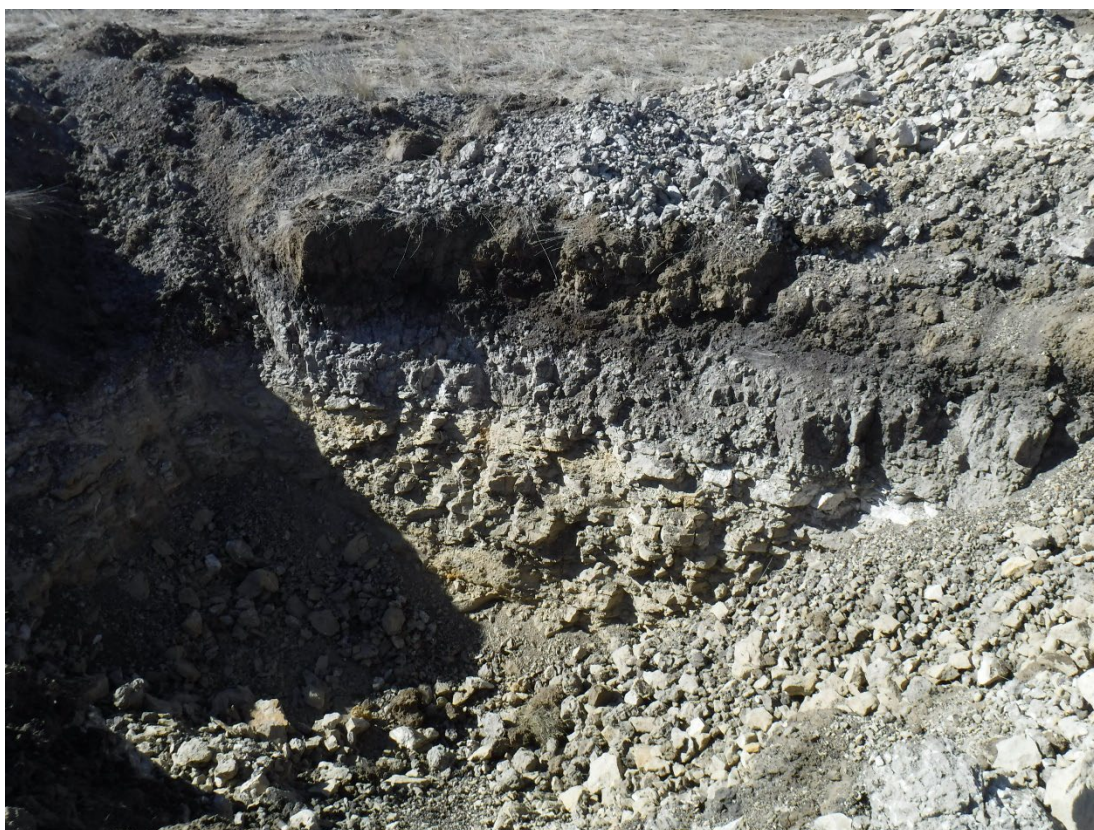
Photo 2: Another pit dug at the site, topsoil loam to weathered bedrock (sandstone)
