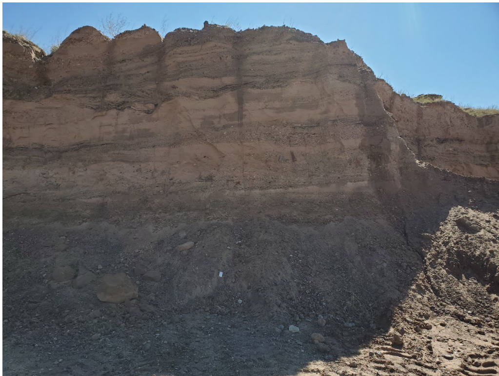
Photo 6: Looking east at the highwall along the northeast side of the permit boundary. The notebook in the photo was used in combination with ImageJ to estimate the highwall height.
