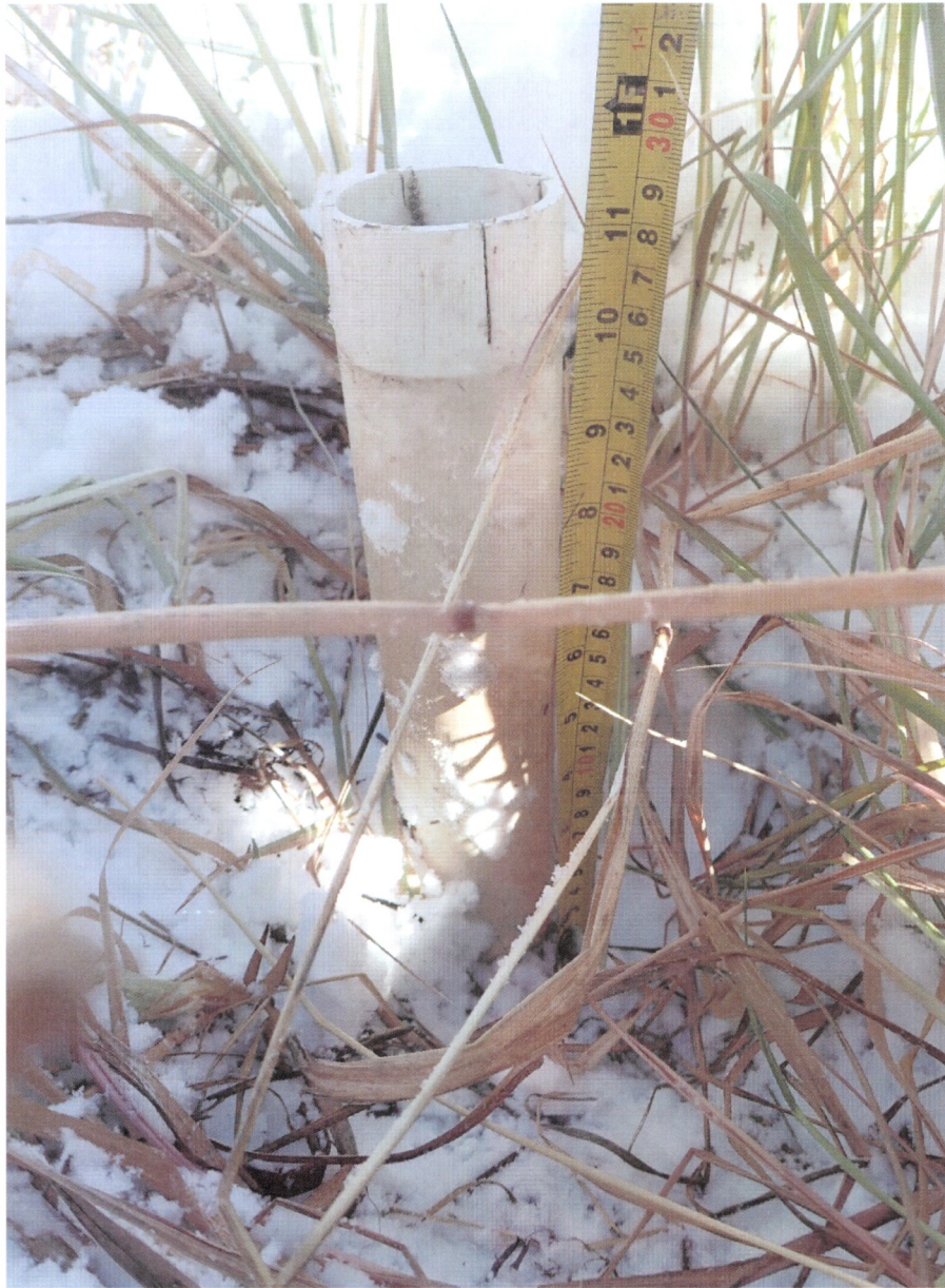
Piezometer GW-3 with casing measurement.
