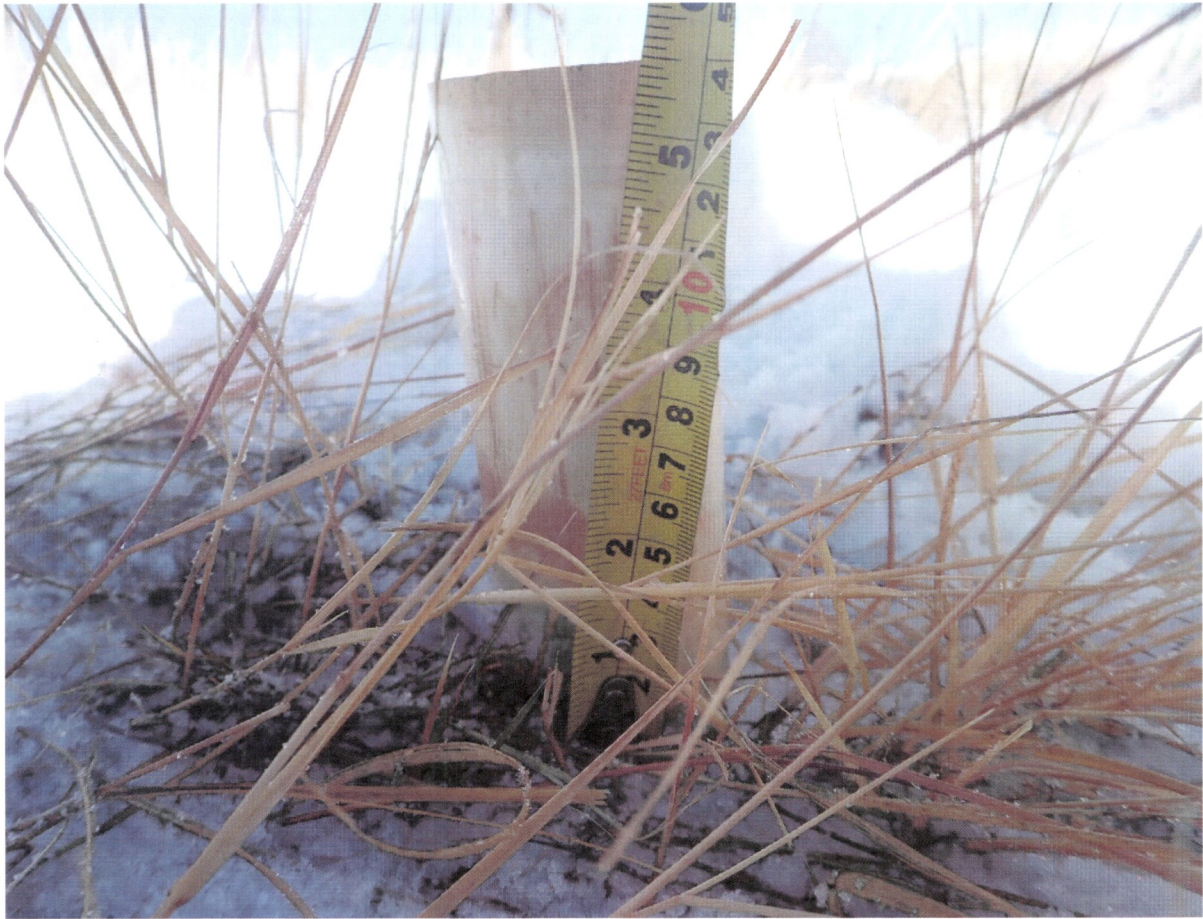
Piezometer GW-1 casing measurement.
