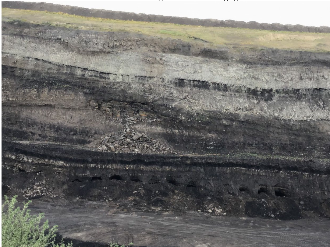
Photo 10: N Pit south highwall rock fall of approximately 20 feet wide.
