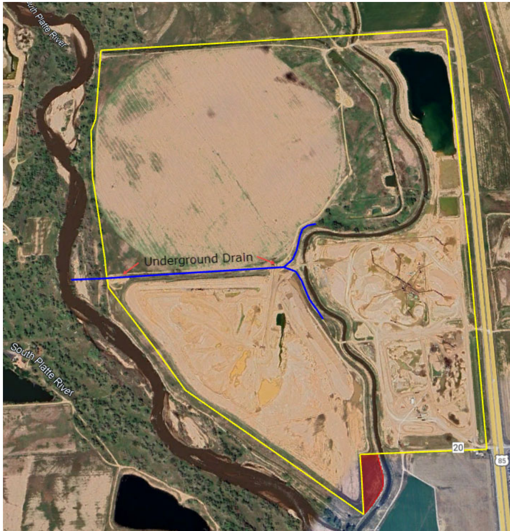
Image 2: Google Imagery showing the approximate permit boundary on the west side of the permit area and the location of the installed groundwater drain (blue line) between the Phase 1 and Phase 2 mining areas. Image dated 9/4/2023.
