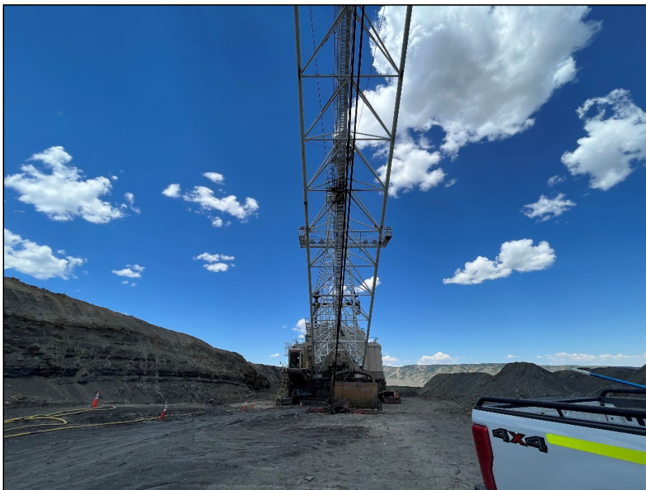
Photo 20: One of two draglines located in Collom Pit, this dragline was inactive at the time of inspection.
