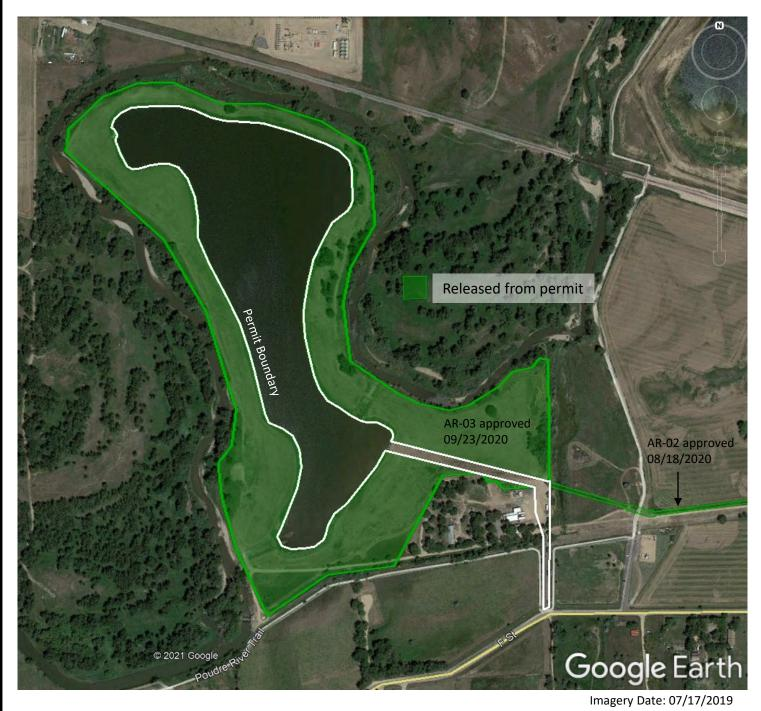
All disturbed areas have been graded, topsoiled and seeded above the water table. All area has been released from the permit, except for the water surface and access to get to the water surface.
