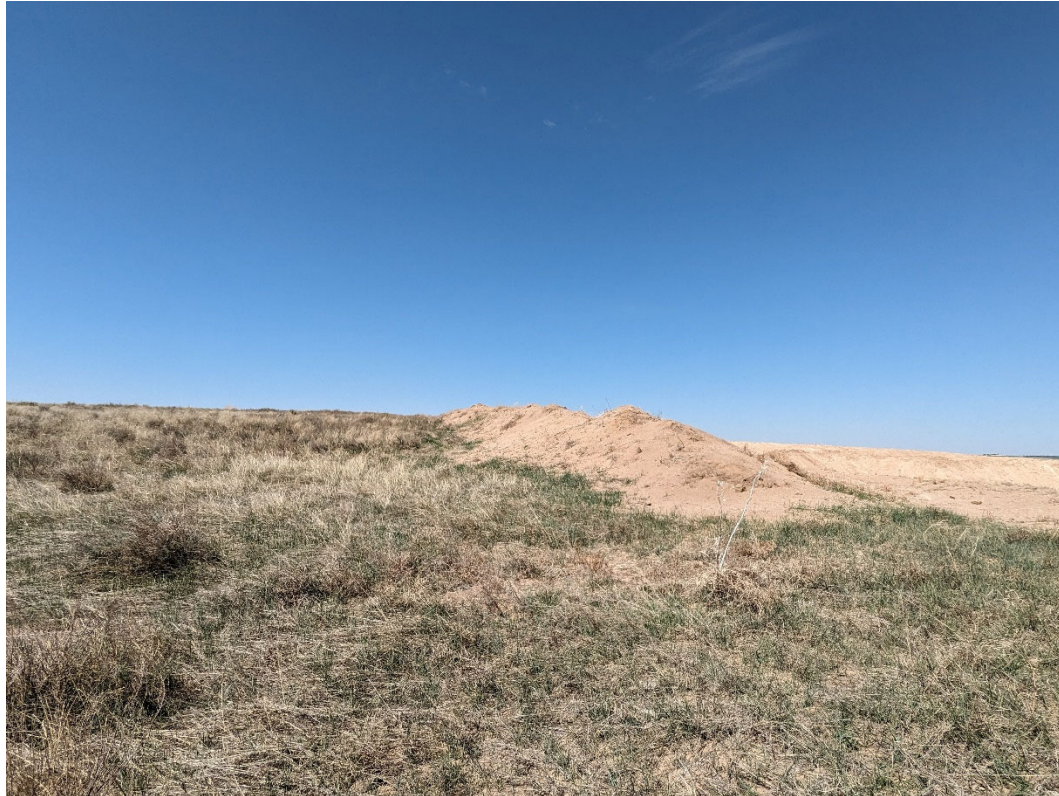
Photo 5: Overburden stored above the southern highwall to prevent water from flowing down into the pit.
