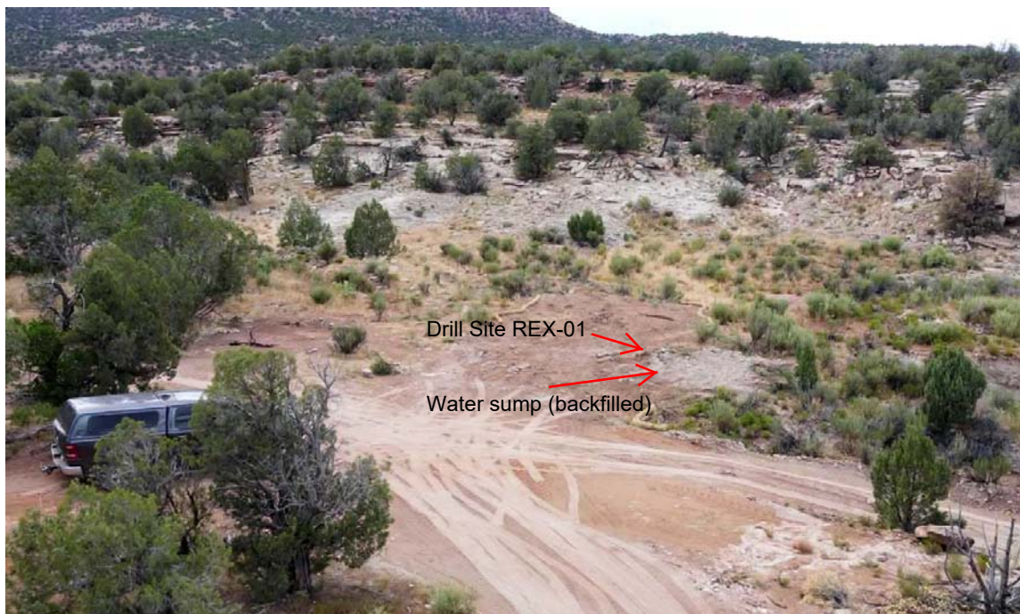
Figure 3: Drone image of REX-01 drill site after scarification and implementation of storm water control measures.
