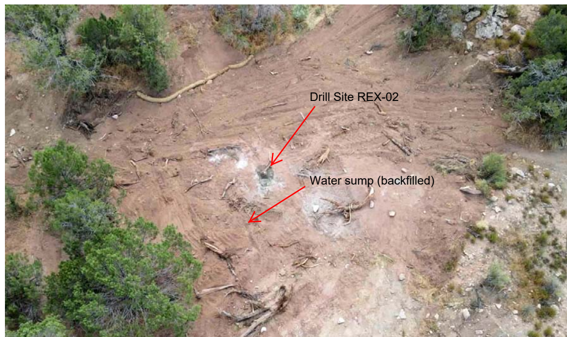
Figure 4: Drone image of drill site REX-02 after scarification and implementation of storm water control measures.
