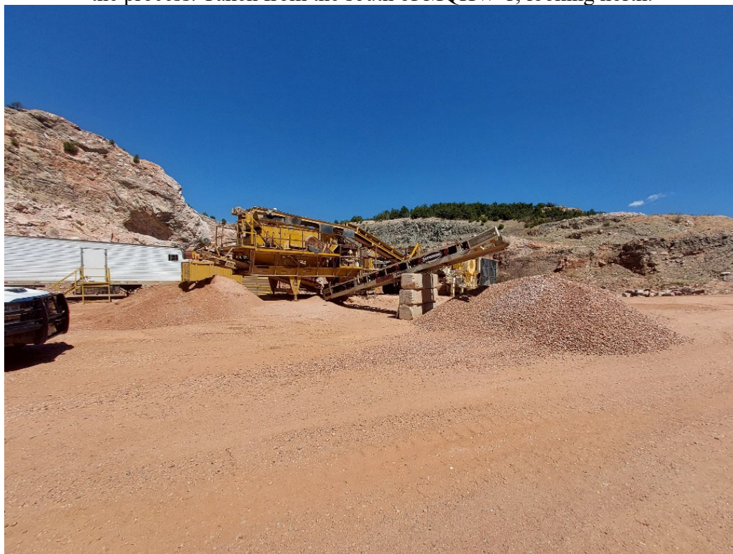
Photo #4: Crusher setup in the MQD-1 Dump area, the small stockpile of processed material can be seen; looking northwest.
