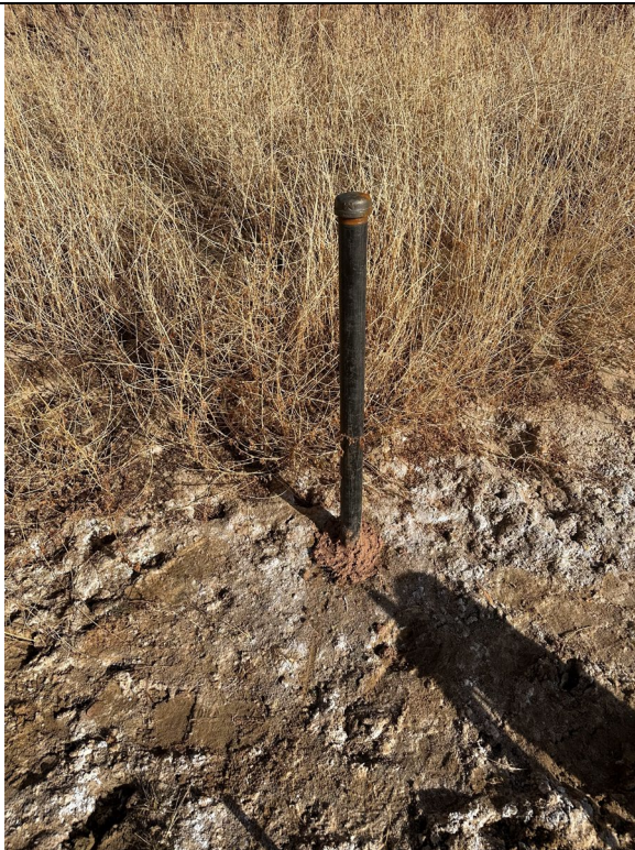
Photo 47: 10/17/2023 Groundwater well installed at the toe of the channel.
