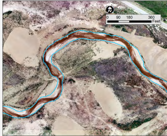
Fig. 10. Drone imagery illustrating the pattern of bar formation that formed after the 2022 flood. The freshly graded Little Joe mitigation site can be seen on the right side of the photograph. The blue line delineates the approximate extent of the inset floodplain in 2023.
