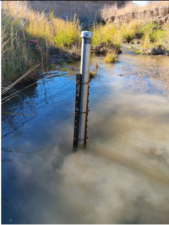
Photo 45: 10/17/2023 Staff gauge installed in the channel thalweg.
