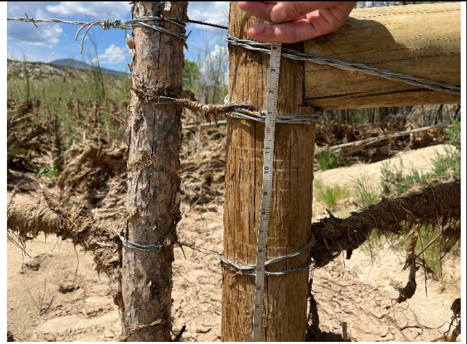
Photo 14: 5/25/23 Height of high flow debris measurement near cross section STA 2+40
