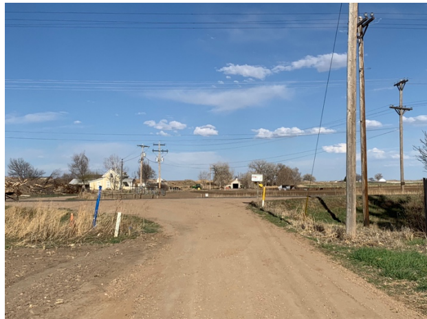
Entrance to right of way with water meter by blue stake water line is buried in the middle of the driveway mailbox and REA power pole on left Yellow pole is gas line marker. White stake marks a culvert running under driveway
