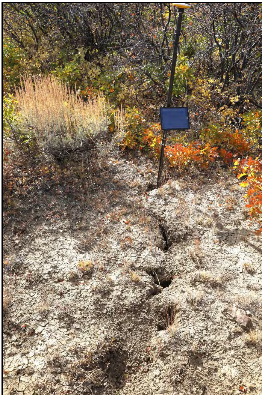
Figure 5. Crack observed along D-D' over Longwall Panel E14 during fall 2023 site visit.
