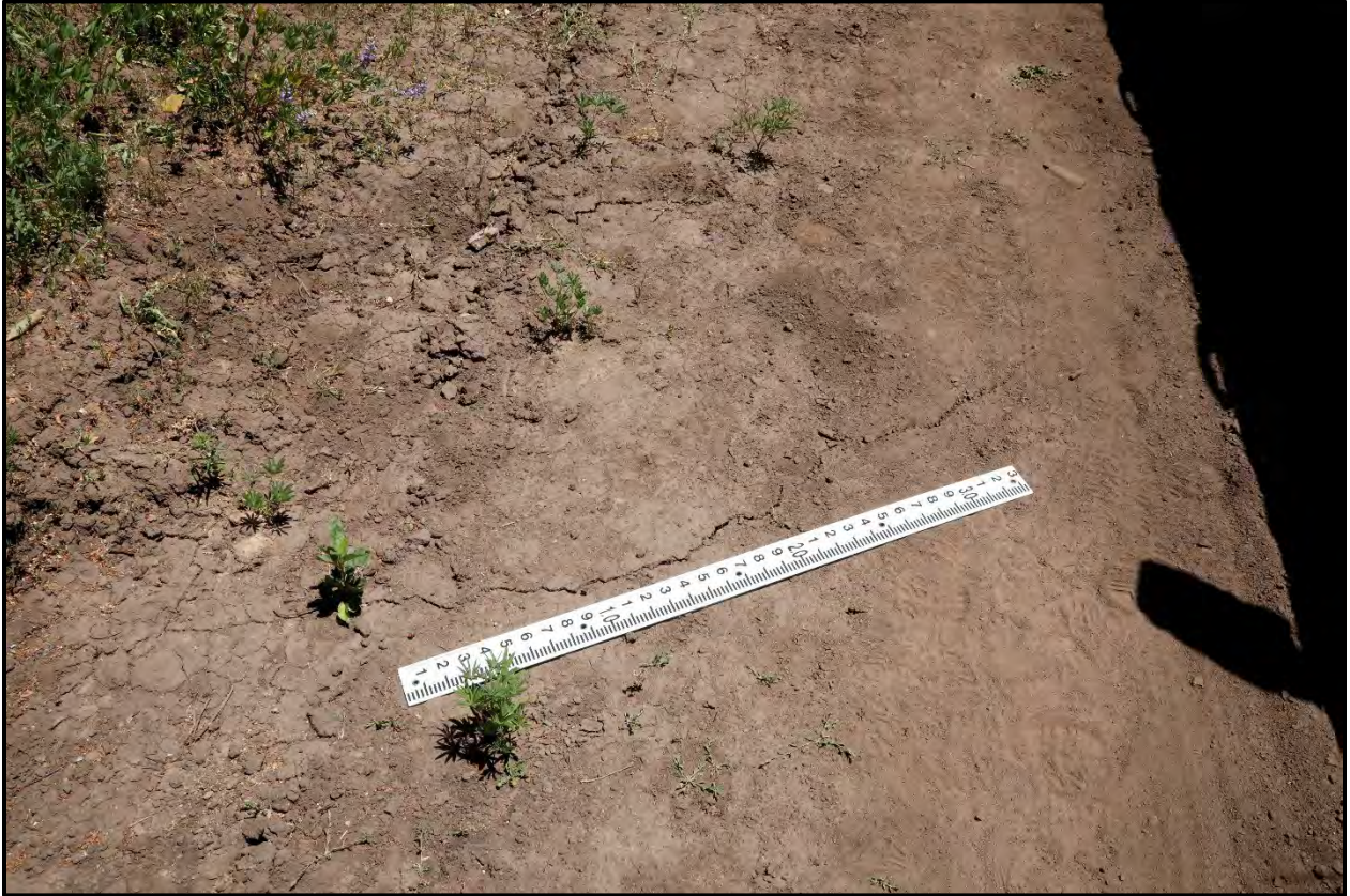
Figure 6: Example of a newly observed crack along the north side of E-seam Longwall Panel SS3 during spring 2023 site visit
