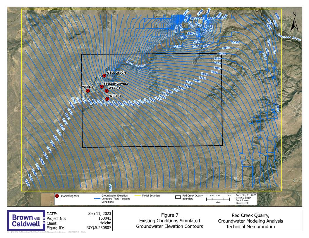
Visual field observations were conducted on Red Creek in December 2022. The steady-state EC model was also calibrated to the visual observations of flow conditions in Red Creek.
