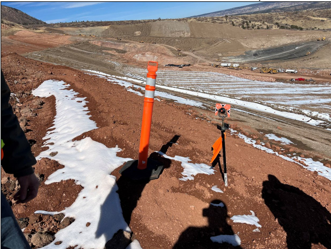
Photo 10: View north of prism 7400-2, material around is loose and easily compacted.
