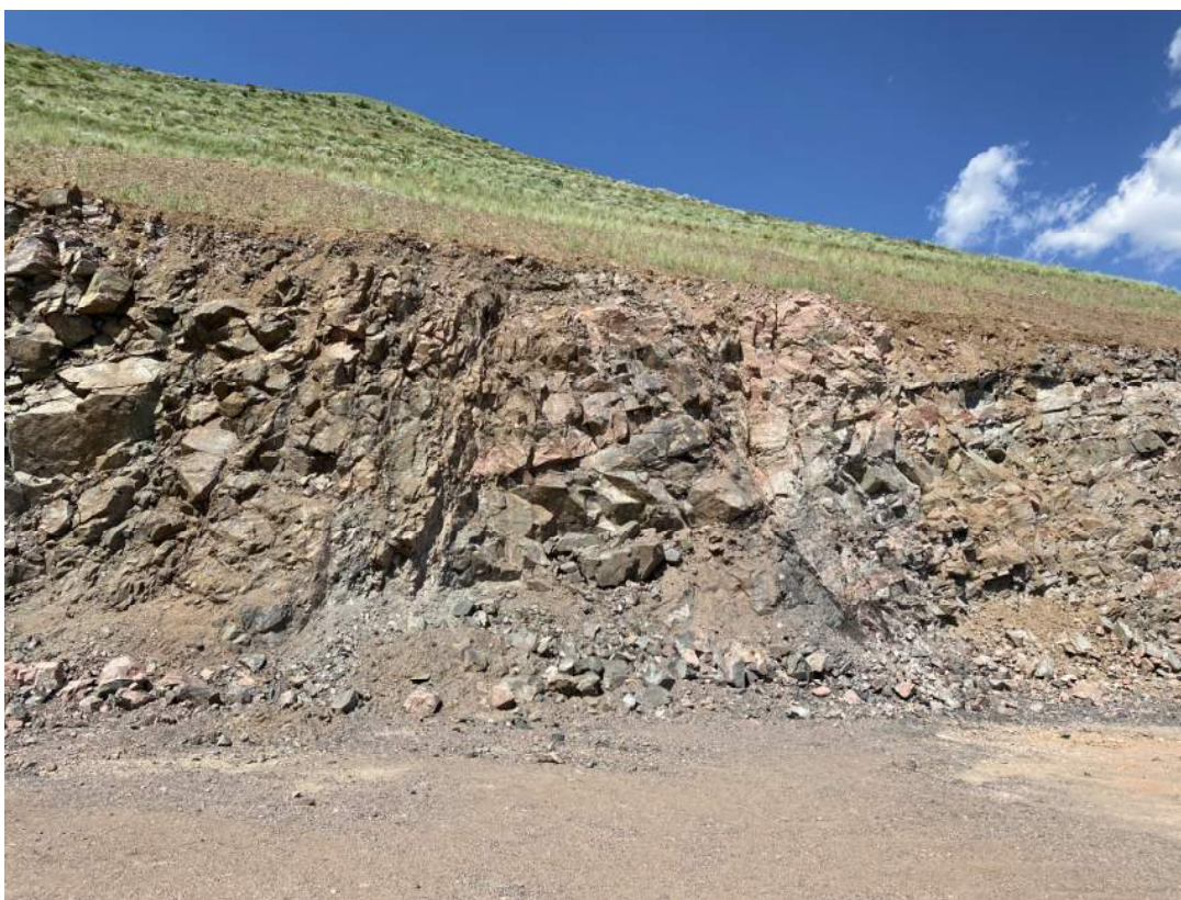
Photo 6: Looking SW at local shear zone in Southern Walls, Bench EL 6440 (June 2023)
