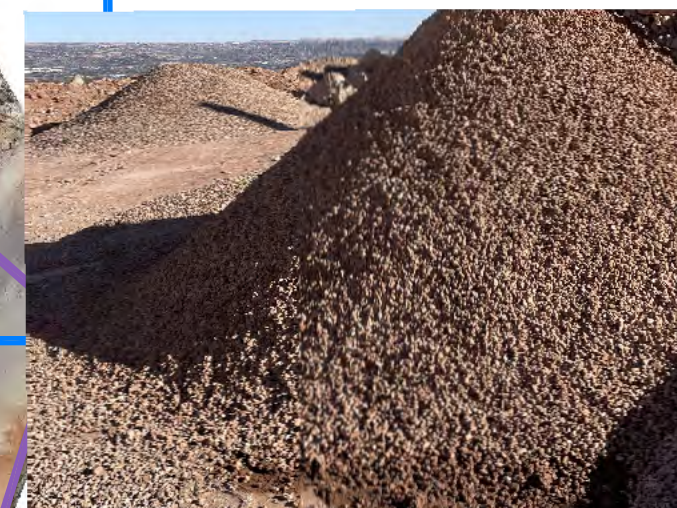
2. Screened gravel stockpile.
