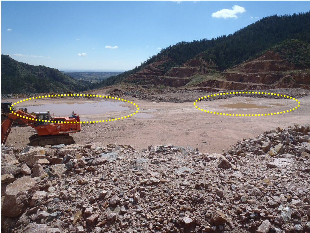
Photo 4. Stormwater ponded on active bench (looking east – highwalls undergoing reclamation beyond).
