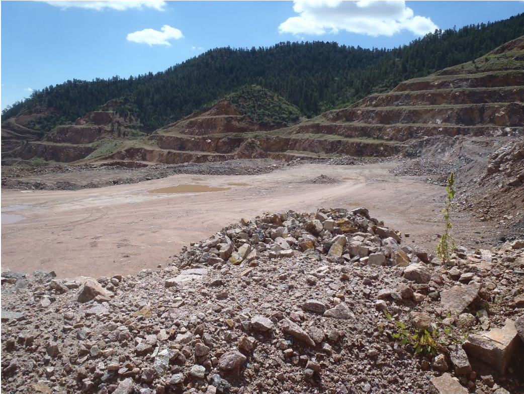
Photo 5. Typical site highwalls before presplitting practice initiated (SW corner).
