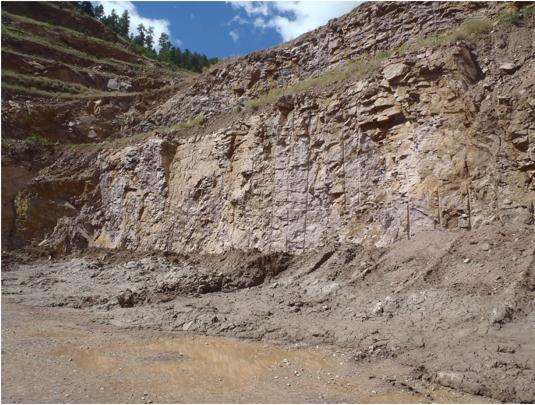
Photo 3. Presplit highwall face with sediment placed at toe (toe of west highwall).
