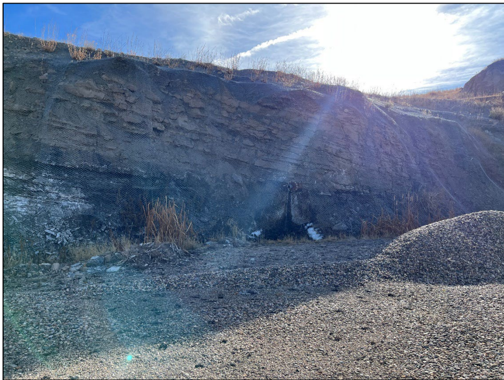
Photo 8: A natural spring leeches from a wall at the portal entries. Ditches capture and carry this water to be pumped back out of the portal area.
