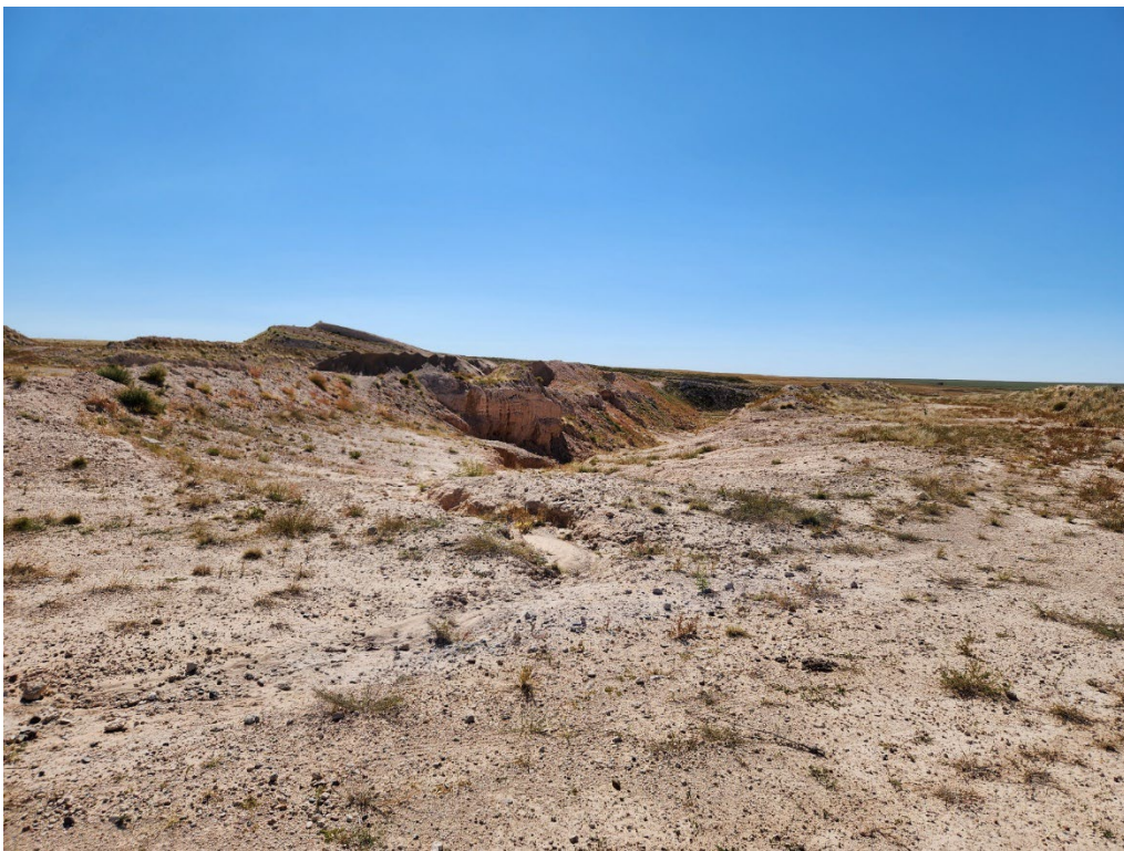
Photo 4. The old mining pit is in the center of the image, looking south. A new mining pit is being excavated to the left. The operator plans to connect these pits by digging out the highwall in between the pits.
