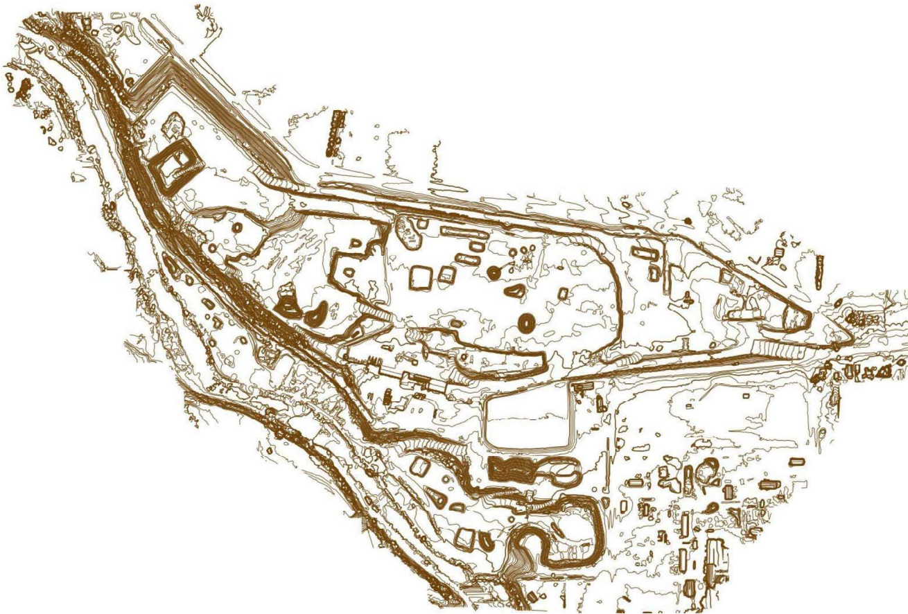
LIDAR contour schematic, August 2023. Note: the entire property drains towards the Arkansas River (lower left).
