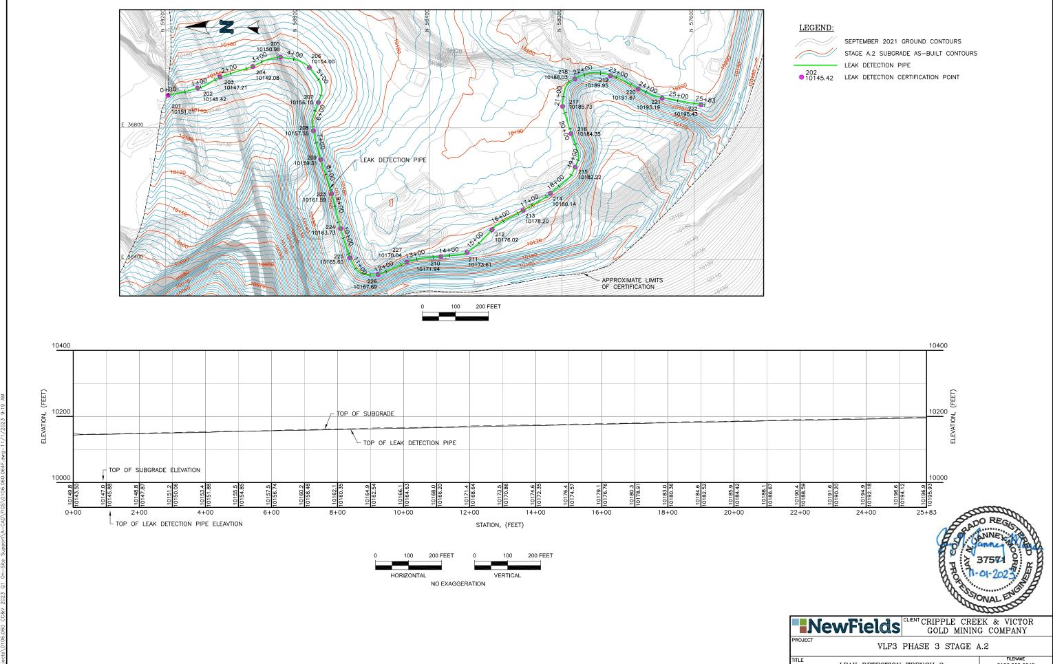
LEAK DETECTION TRENCH 2 AS-BUILT PLAN AND PROFILE
