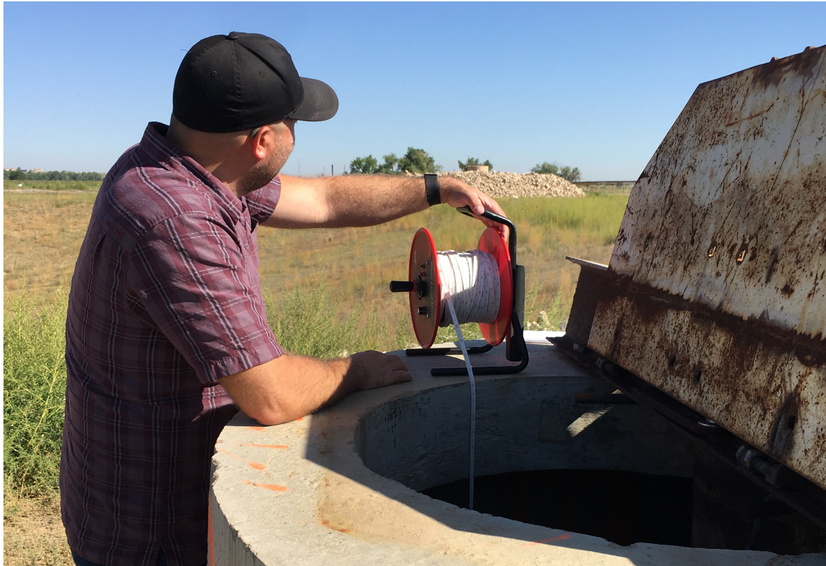
Figure 6 - Reservoir water surface measurement from wet well.
