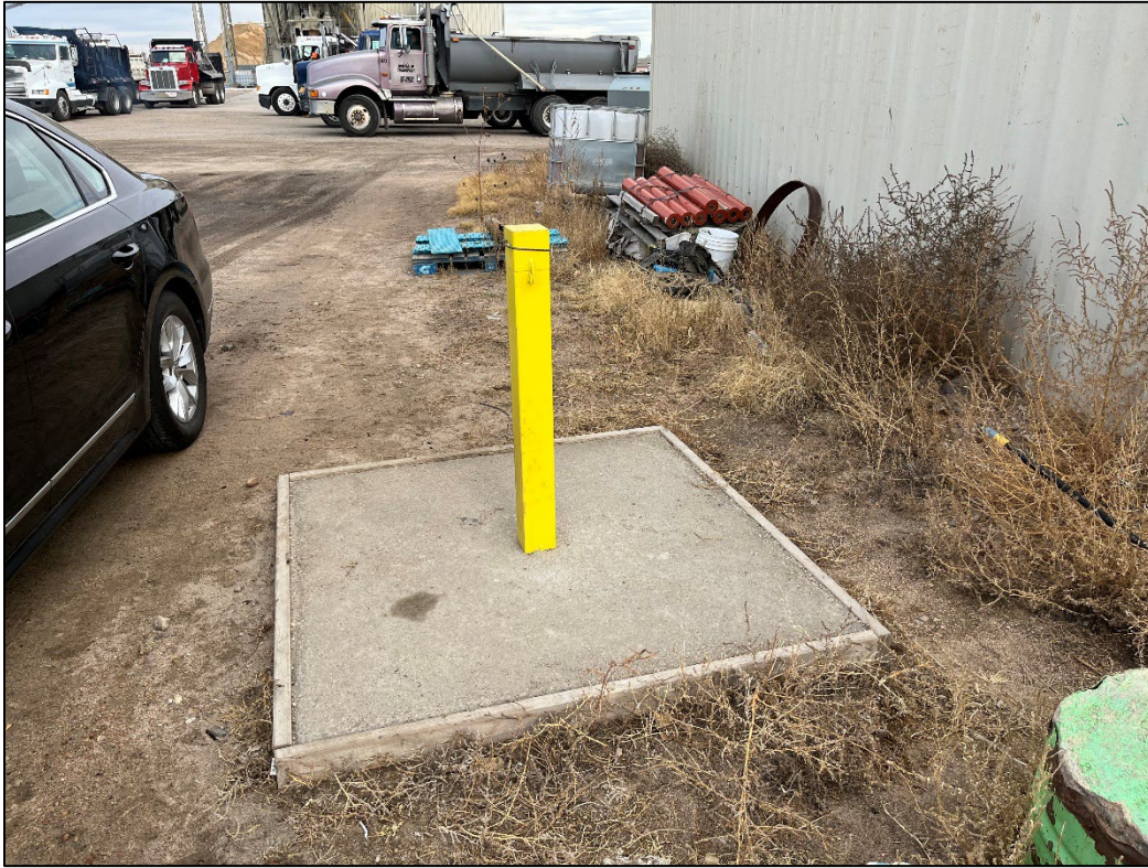
Photo 7: One of two monitoring wells replaced on the eastern side of the permit.
