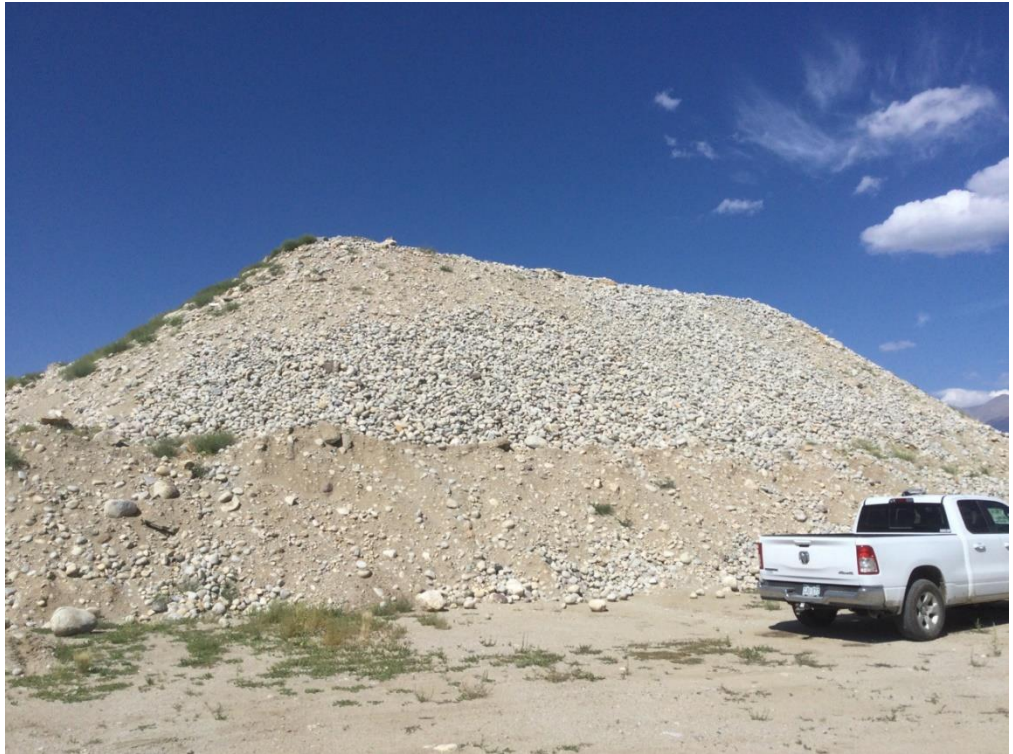
Photo 7. Stockpile 24 Reject cobble, due to gradation and appearance, blended through crusher with Stockpile 23 to make Road Base
