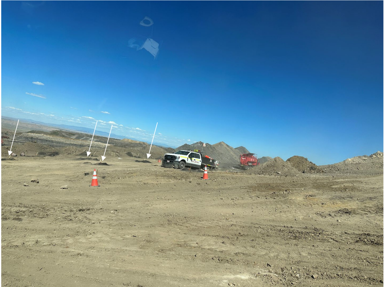
Figure 3 - The operator preparing an overburden blast. Note the blastholes (white arrows).
