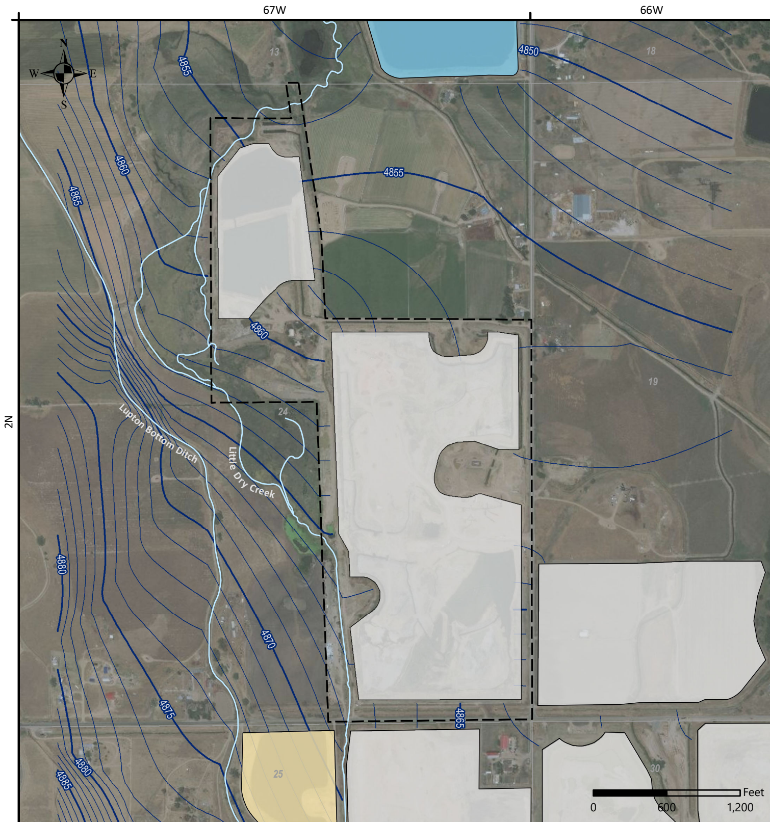
Figure 12 NCCI Pit - Summer Water Table with Liner (no drain)
