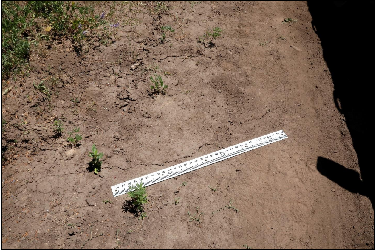
Figure 5: Example of a newly observed crack along the north side of E-seam Longwall Panel SS3
