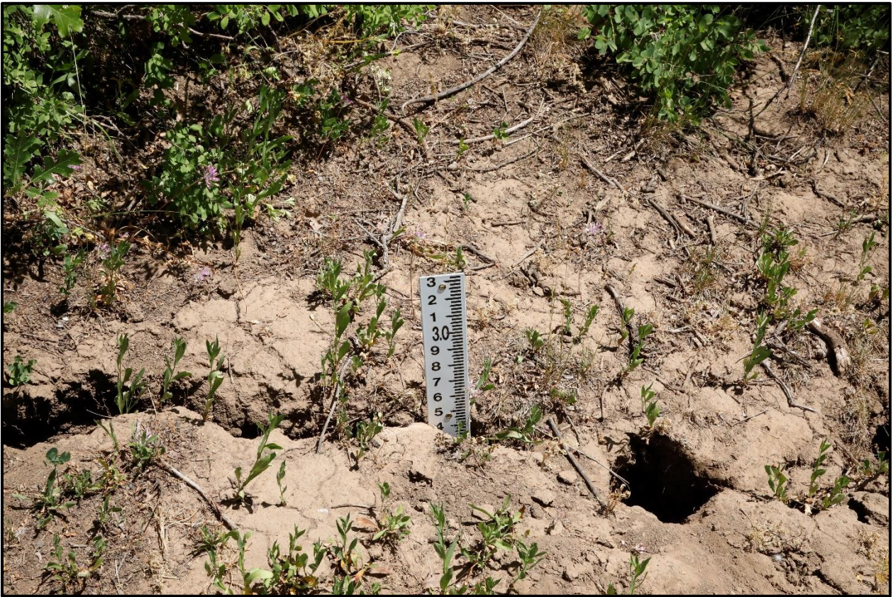
Figure 4: The largest of the cracks at Location 2, south of the across road on Traverse C-C' during spring 2023 visit.
