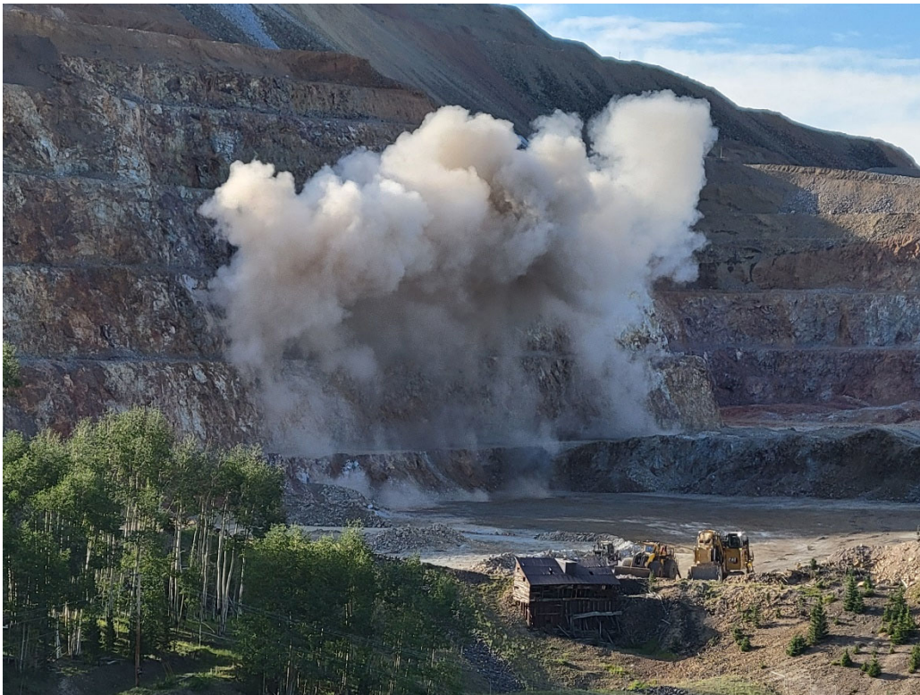
Photo 2. Pre-split blast at Schist Island. Looking east across Highway 37 from the overlook at the Heritage Center.
