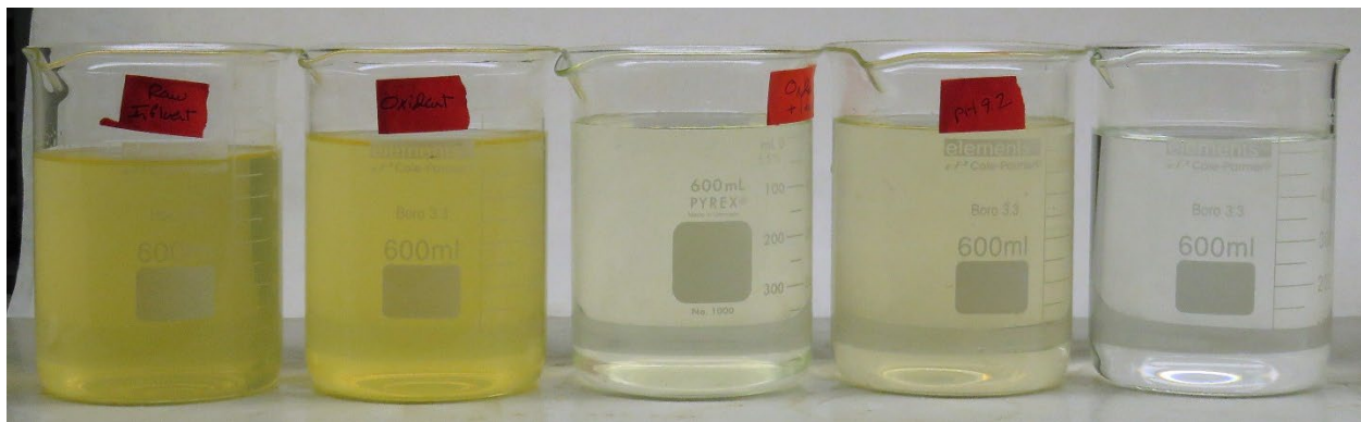
Figure 4. Bulldog mine treated samples at initial sample collection from left to right: influent, oxidant > 1 \mu m, pH 9.2, pH 9.2 > 1 \mu m
