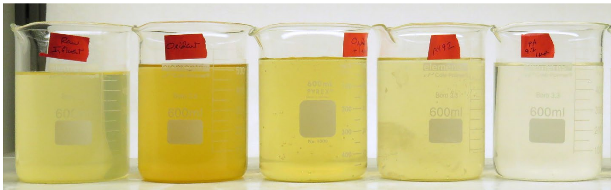
Figure 5. Bulldog mine treated samples 6 hours after initial testing from left to right: influent, oxidant > 1 \mu m, pH 9.2, pH 9.2 > 1 \mu m, pH 6.8
