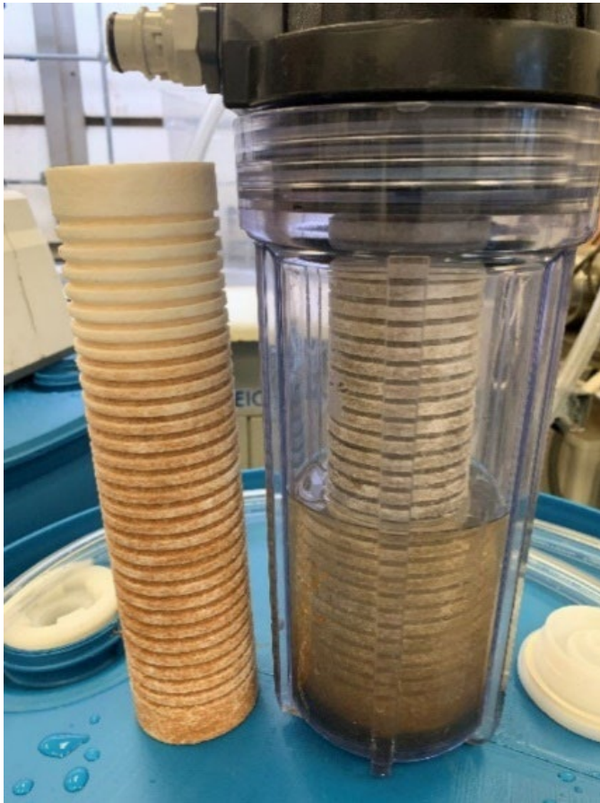
Figure 7. Filters after testing, Oxidant > 1 \mu m (left), pH 9.2 > 1 \mu m (right)
