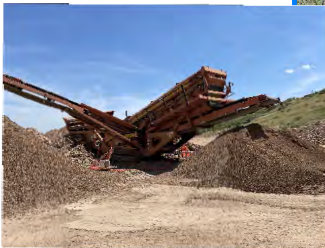
8. Astec near pit floor processing riprap.
