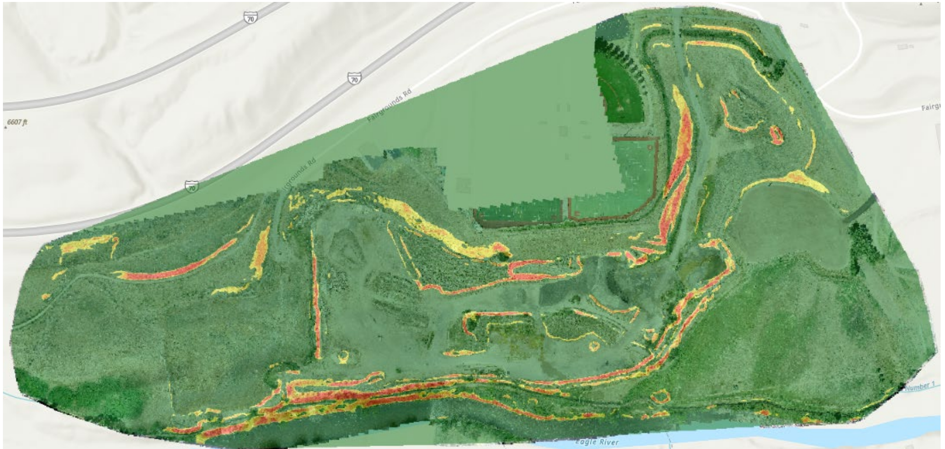
Figure 5: Screenshot from ArcGIS Online showing orthomosaic of whole of surveyed area, overlaid with slope raster.
