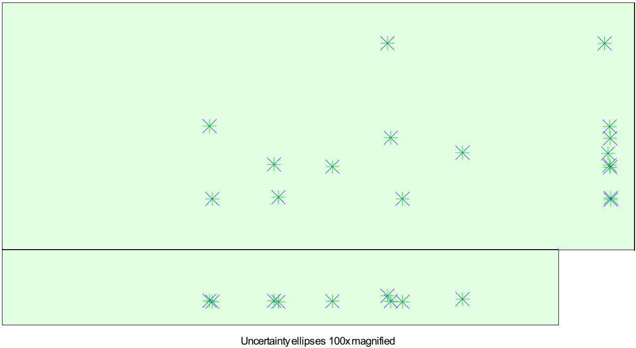
Figure 3: Offset between initial (blue dots) and computed (green dots) image positions as well as the offset between the GCPs initial positions (blue crosses) and their computed positions (green crosses) in the top-view (XY plane), front-view (XZ plane), and side-view (YZ plane). Red dots indicate disabled or uncalibrated images. Dark green ellipses indicate the absolute position uncertainty of the bundle block adjustment result.
