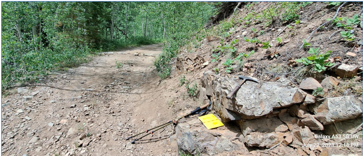
Figure 3: Lowest in-place rock outcrop observed during inspection. The rock appeared to be hydrothermally altered, intermediate composition igneous intrusive with sulfide mineralization visible on fresh surfaces which appeared to include pyrite, and possible galena and chalcopyrite. Hammer for scale. View is looking north at location B on the map.
