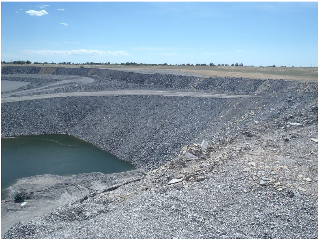
Photo 2. Backfilled SE portion of active quarry (looking SE).
