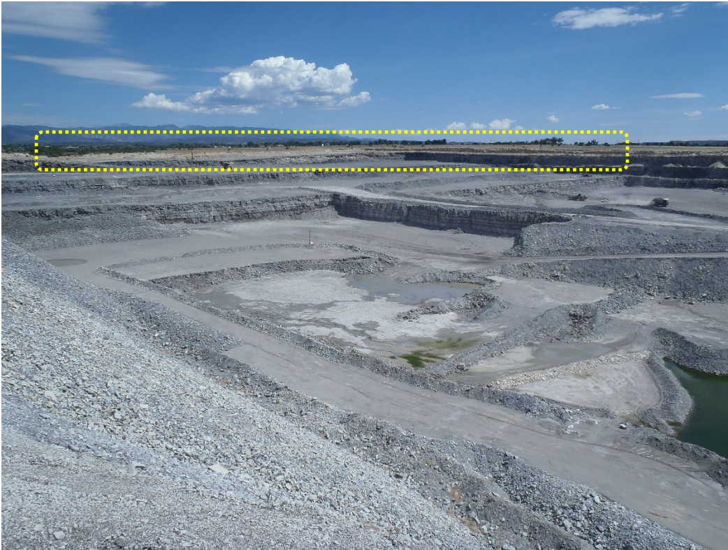
Photo 3. Stripped overburden on north edge of quarry (circled) (looking NE; Note wide benches).
