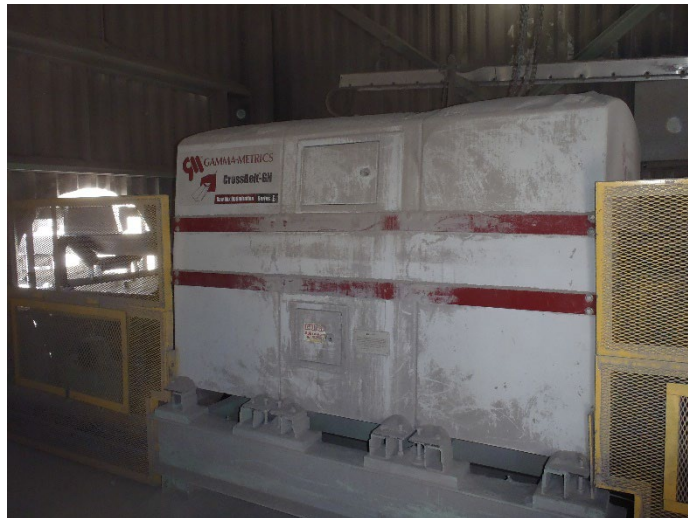
Gamma-Metrics Analyzer (indoors, radioactive material).
