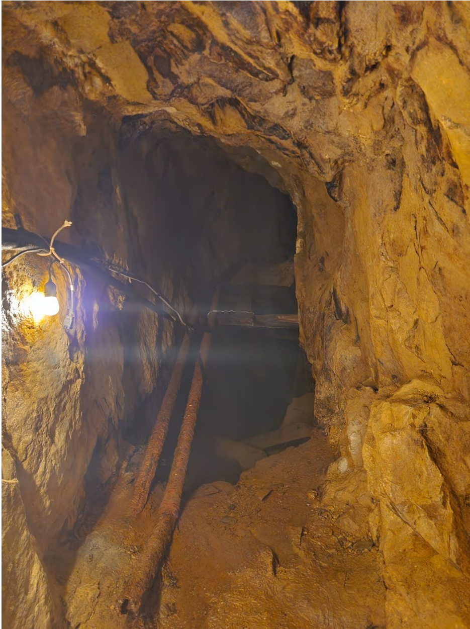
Winze location showing \frac{3}{4} " and 1\frac{1}{4} " Piping
