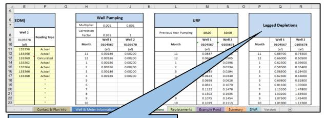
Lagged Depletions should be calculated utilizing the Well Pumping data and the lagging method established by the relevant decree or SWSP (Stream depletion Factors or Glover Parameters).
