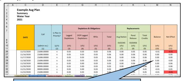
The Balance column is the balance of Replacements and actual Depletions/Obligations regardless of whether the plan is in or out of priority. It is calculated by subtracting Depletions and Obligations from Replacements.
