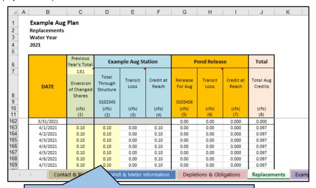
Input information should be shaded differently than the calculated (cells with formulas) cells. Please provide a legend with the color/shading scheme.
