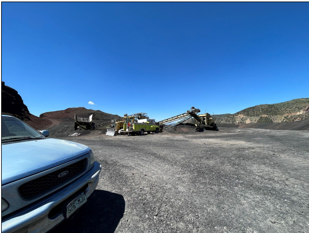
Photo 14: Two screeners are kept onsite to sort material into four different sizes.
