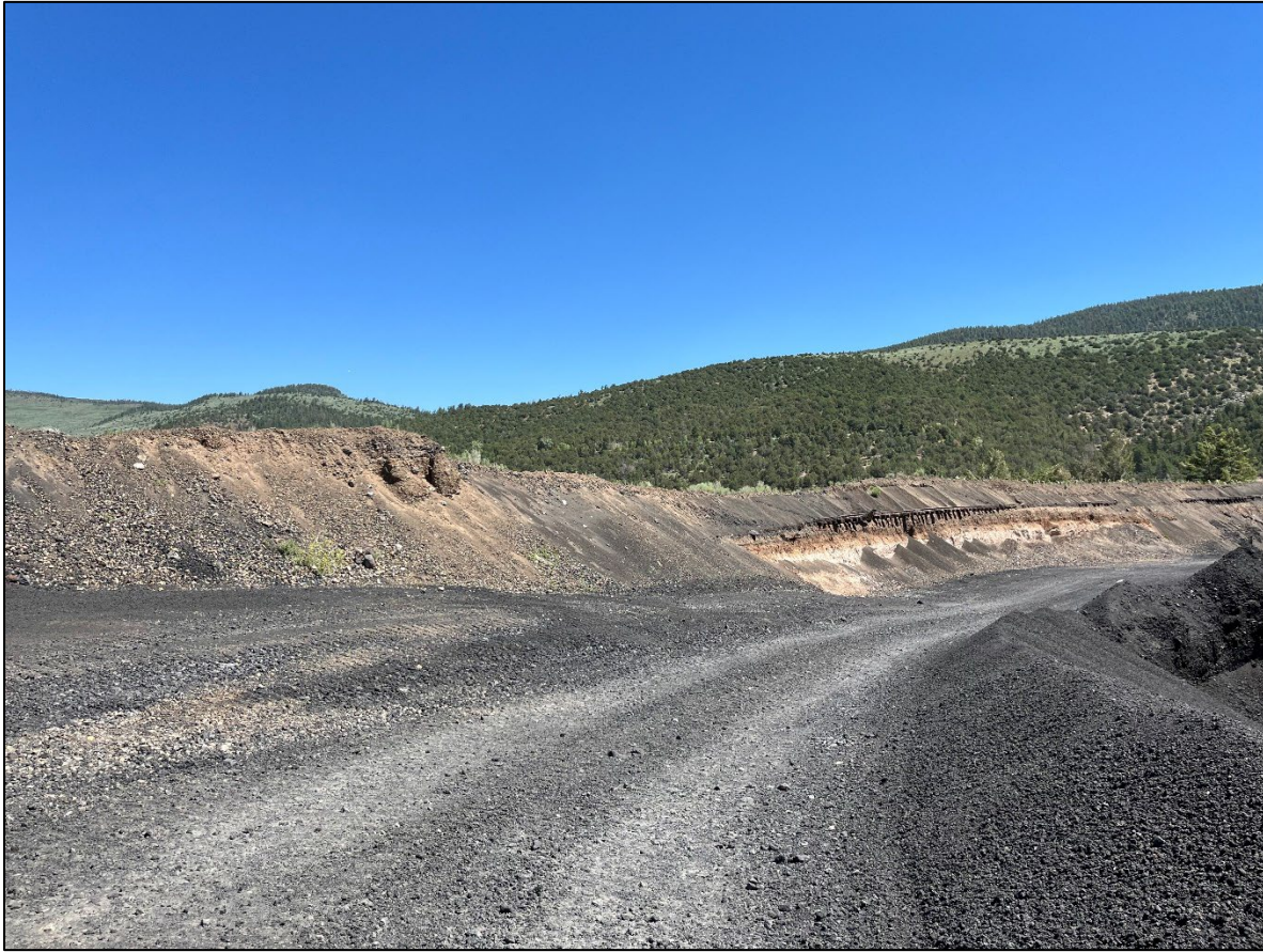
Photo 13: Road down into the active mining area, overburden material is stockpiled along the northern pit edge.
