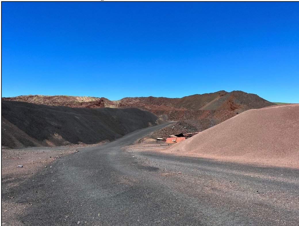
Figure 10: View west of the volcanic crater and various stockpiles, this area is being backfilled contemporaneously as mining progresses.
