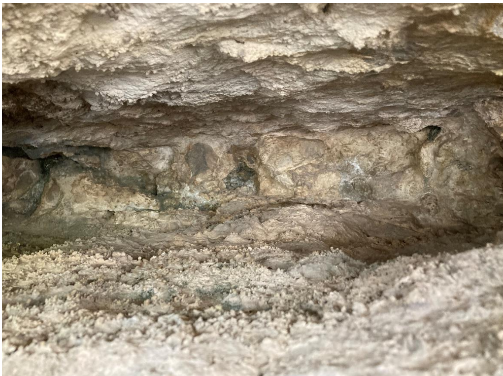
Photo 11 and 12: Interbed material exposed at the East Face is a weak, cemented mudstone with clasts of limestone. (4/14/23 Photos# 2028 and 2025)
