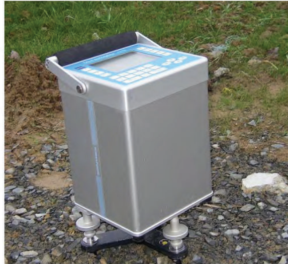
Figure 9: Photo showing gravimeter. The gravimeter is approximately 12 inches by 8.5 inches.
