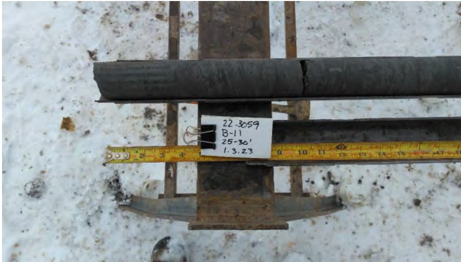
Photo 53. Boring B-11 at 30 to 31 feet. Depth interval in photo is incorrect.
