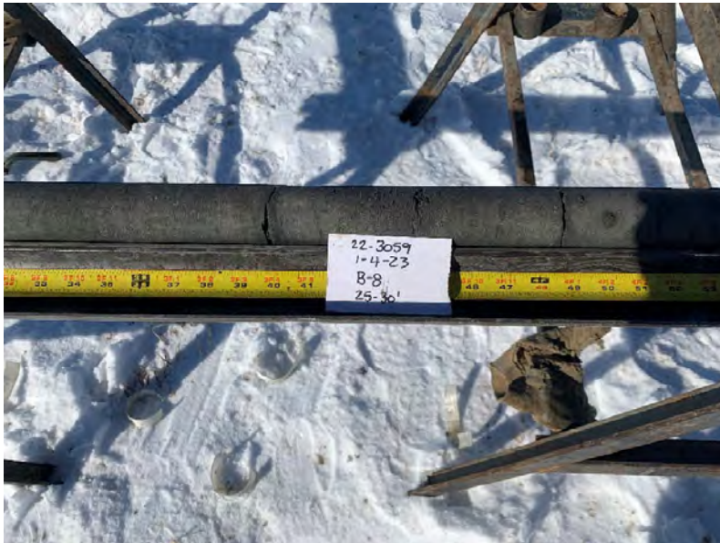
Photo 37. Boring B-8 at 28 to 29 feet.
