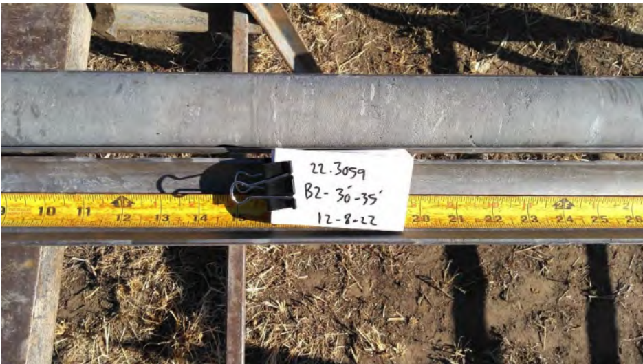
Photo 12. Boring B-2 at 31 to 32 feet.
