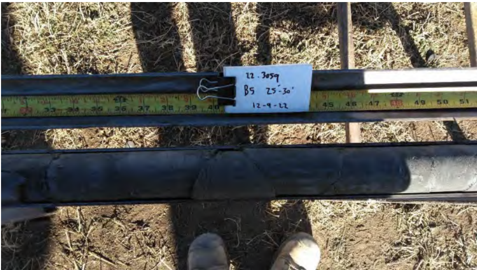
Photo 23. Boring B-5 at 28 to 29 feet.
