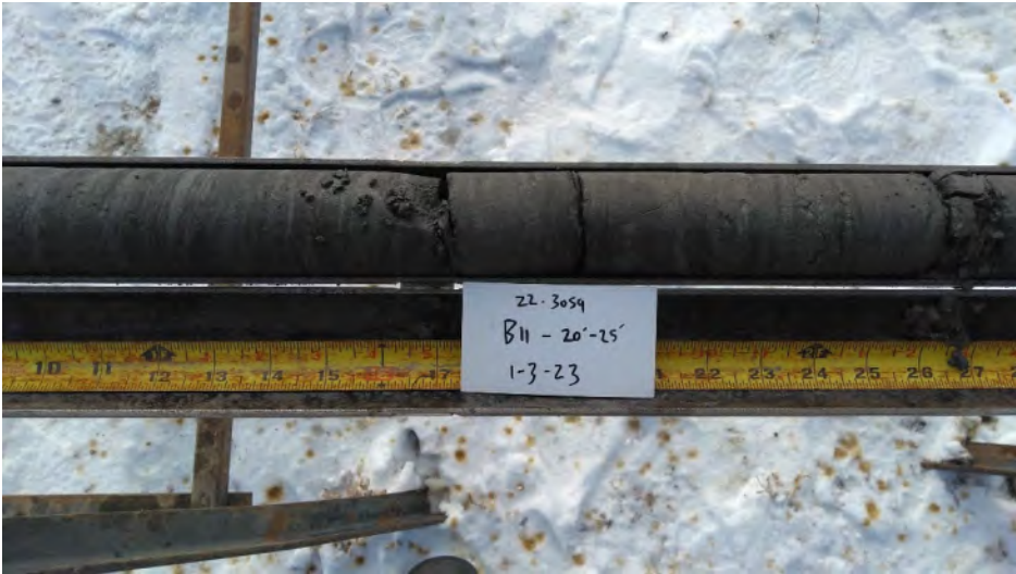
Photo 45. Boring B-11 at 21 to 22 feet.
