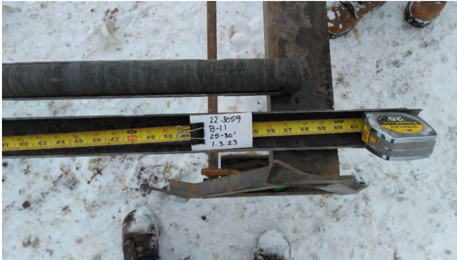
Photo 57. Boring B-11 at 34 to 35 feet. Depth interval in photo is incorrect.
