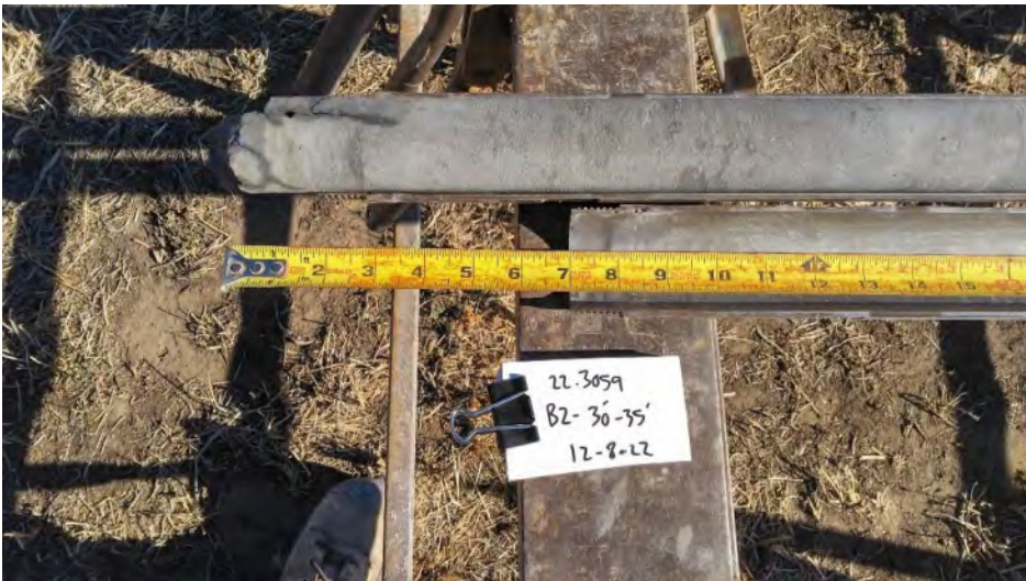
Photo 11. Boring B-2 at 30 to 31 feet.
