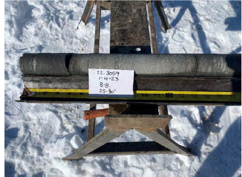
Photo 34. Boring B-8 at 25 to 26 feet.
