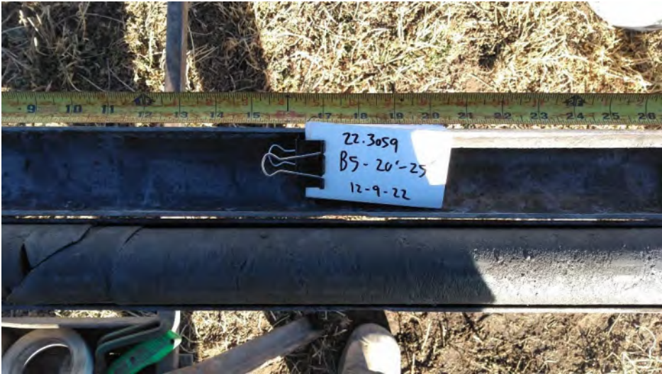
Photo 17. Boring B-5 at 21 to 22 feet.
