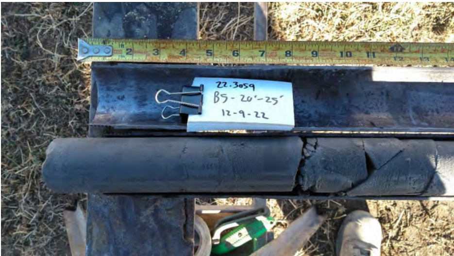
Photo 16. Boring B-5 at 20 to 21 feet.
