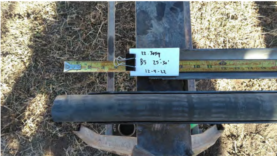
Photo 20. Boring B-5 at 25 to 26 feet.
