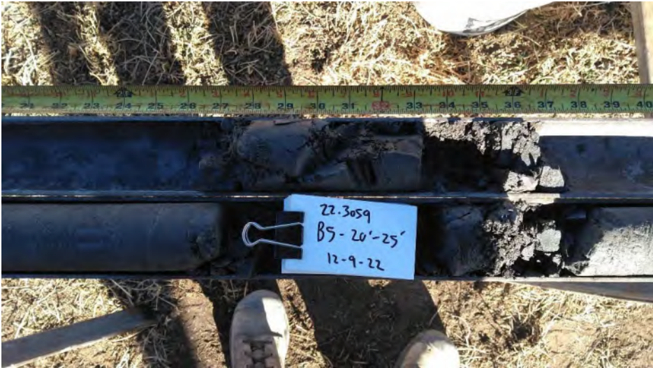
Photo 18. Boring B-5 at 22 to 23 feet.
