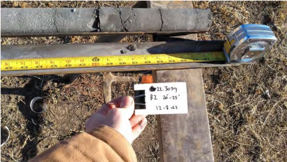
Photo 5. Boring B-2 at 24 to 25 feet.
