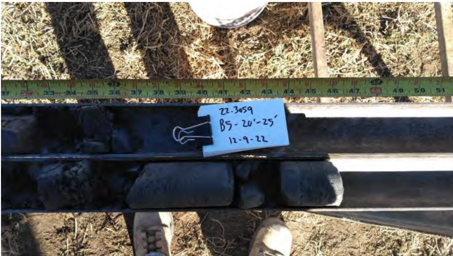
Photo 19. Boring B-5 at 23 to 24 feet.
