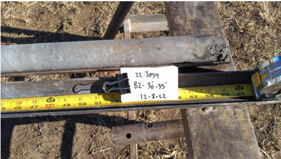
Photo 15. Boring B-2 at 34 to 35 feet.
