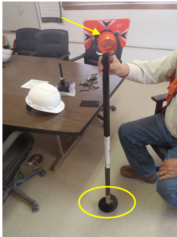
Photo 5. New auger-based prism (auger at base, prism on top).
