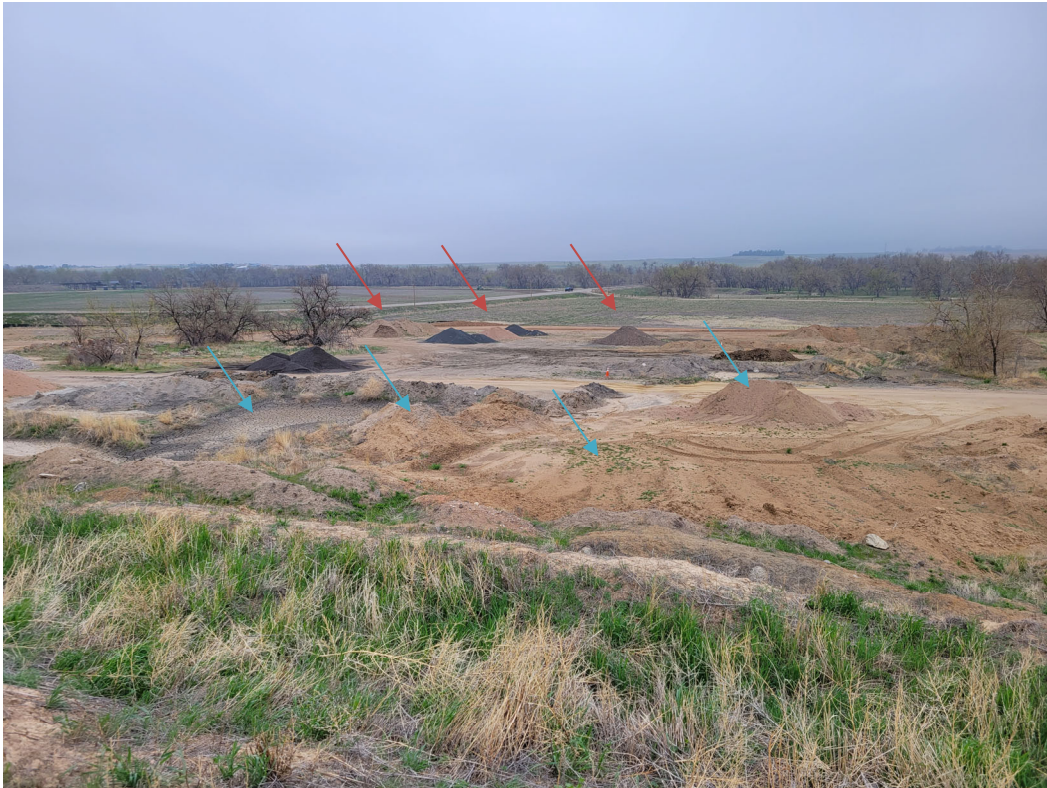
Photo 1. Looking northeast from the western highwall across the mining area. Landscaping and mining material stockpiles in the background (red arrows). Slurry basins and clay berms and stockpiles in the foreground (blue arrows).
