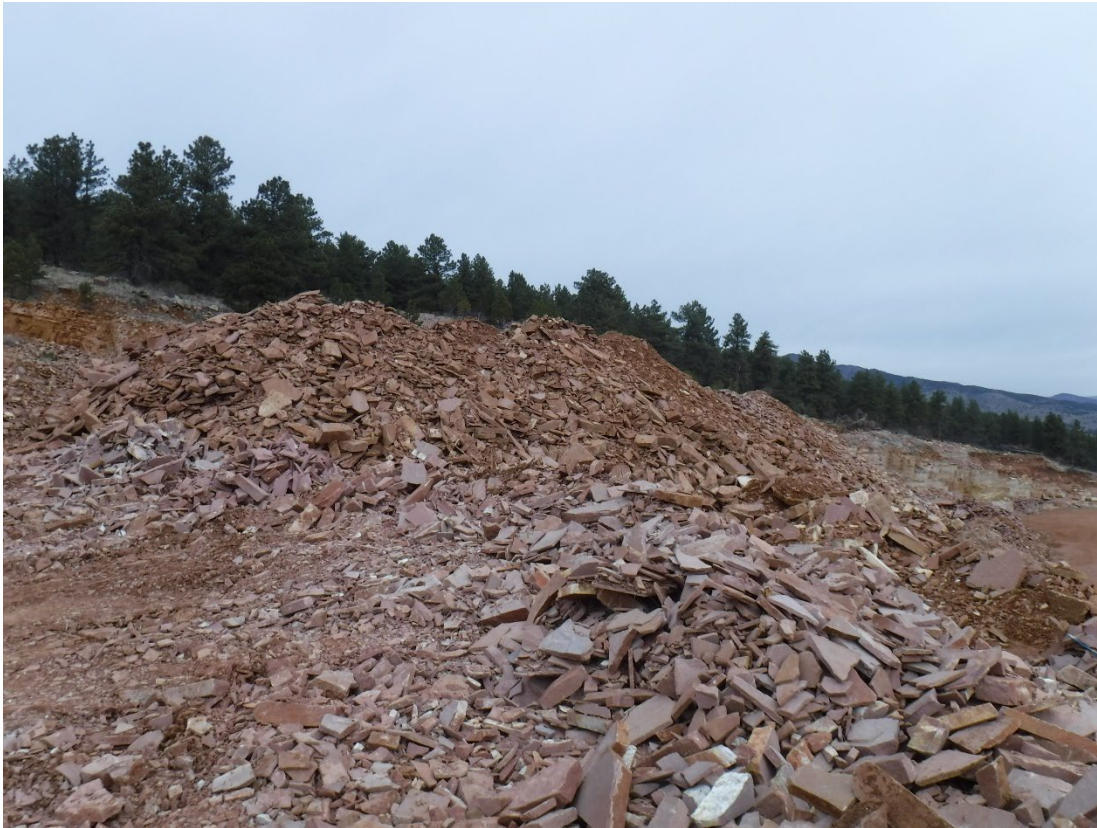
Photo 13: Typical overburden and waste rock stockpiles positioned to be pushed down into pits
