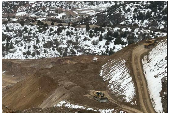
Photo 4 – Looking South to South Quarry from top of West Quarry at dozer and haul truck placing material for reclamation of mined face.
