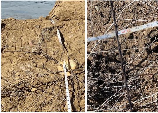
Location 1 Highwall edge to the fence is 14' 2" From the Highwall edge to the road is 21'
