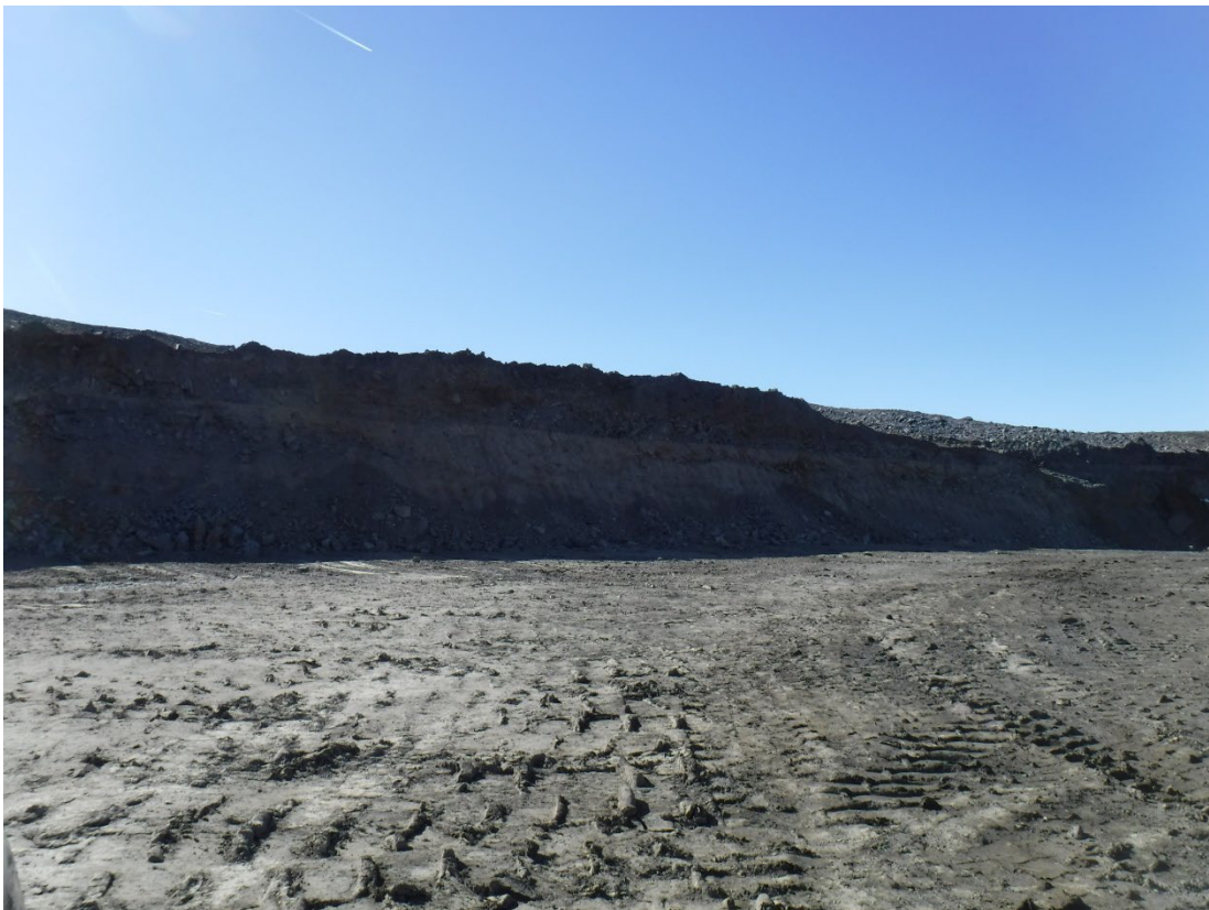
Photo 2: A view of the overburden stockpile face being used for backfill
