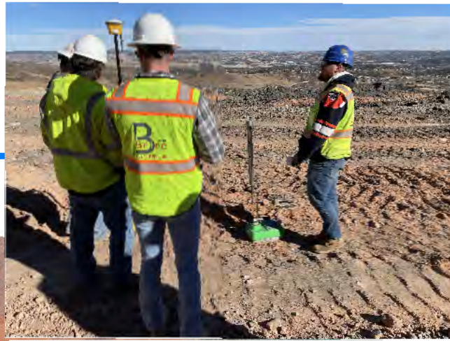
4. Nuclear gauge testing on compacted floor
