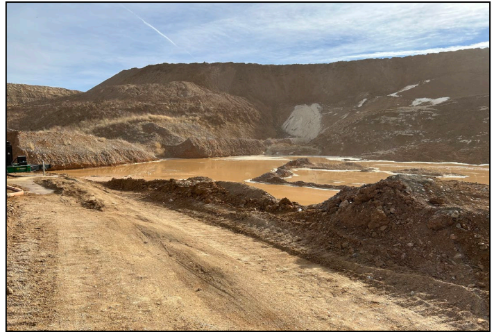
Photo 2 – SE corner of operational mining cell. Water in photo is a process water pond - no groundwater has been exposed at this site.
