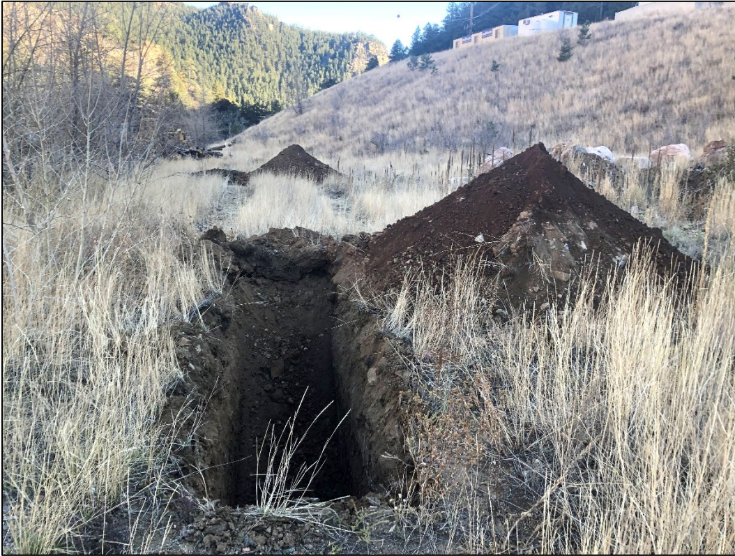
Photo 5. View looking southeast at westernmost soil test pit excavated near base of mesa.
