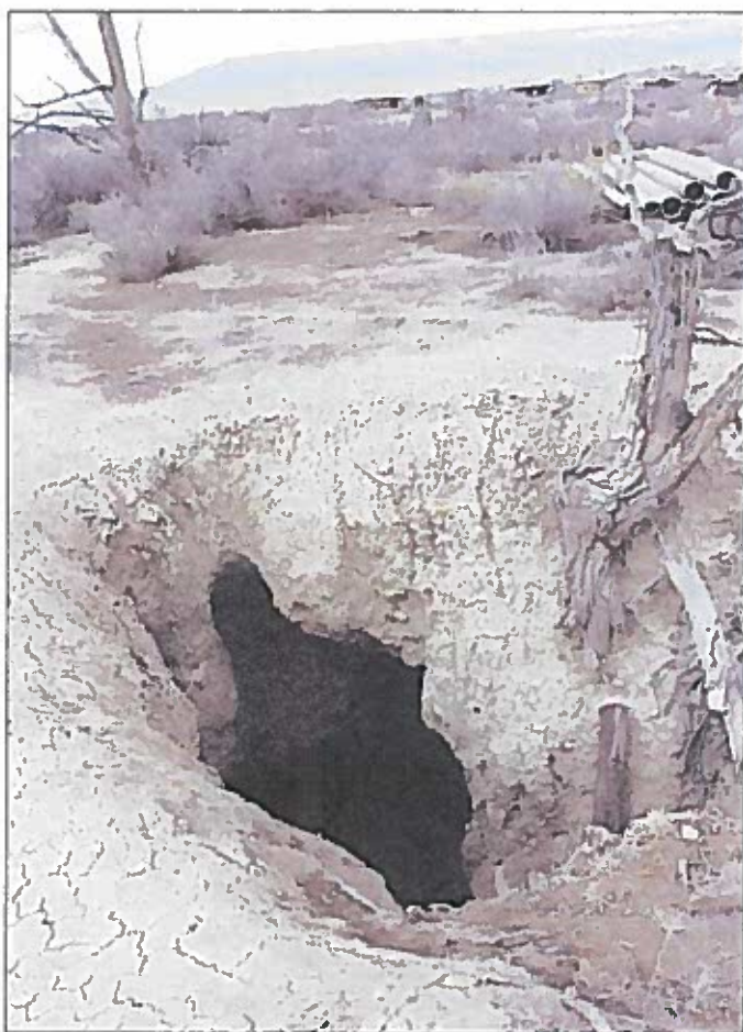
Figure 3-6. Sinkhole and cavern formation due to soil dispersion, piping, and void collapse along Loutsenhizer Arroyo, north of Montrose.
