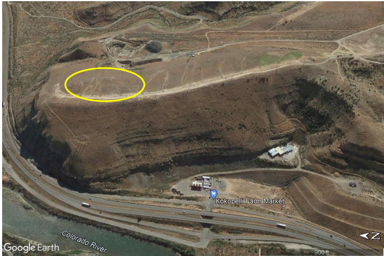
Figure 2. Oblique GE image of linear gravel-capped mesa remnant. Note lateral irrigation ditches on surface. Area of piping/soil dissolution approximated by yellow oval.
