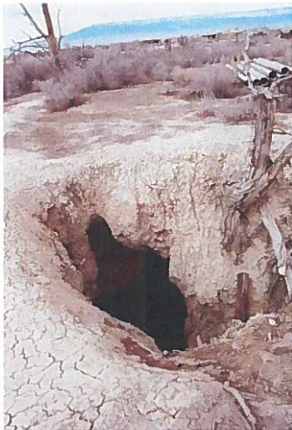
Piping-void surface collapse near Loutsenhizer Arroyo east of Olathe.
