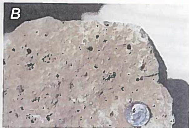
Figure 3-3. Visible, macroscopic voids in collapsible soils. A, A sandy-silt soil in which the primary voids were created at the time of deposition. B, A more clayey soil with secondary voids formed by microdissolution and biogenic activity.
